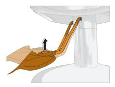
To unlock it, press on the pedal
